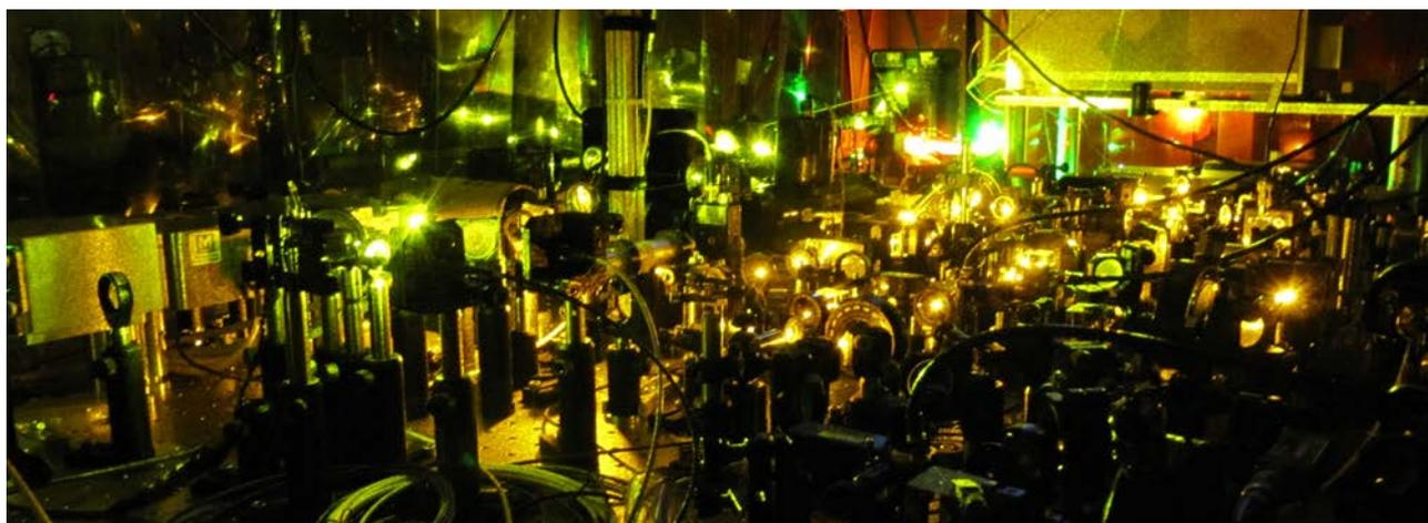
A usual day in my lab starts by switching on numerous computers, power supplies, electronics boxes, and lasers. A remarkable number of devices have to play together in order to create what presumably is the coldest matter in the universe. Our experimental apparatus is capable to bring the movements of atoms almost to a halt, cooling them to the
